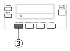
You can give your very dirty laundry a prewash prior to the main wash by using this additional function. When using this function, you should put detergent in the front washing compartment of the detergent drawer.
